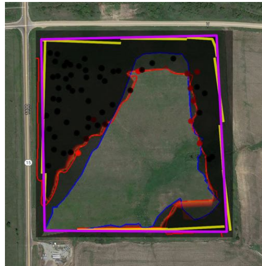
Fig. 11: An example comparing the simulated fire with a participant's corrections (red front) to the actual fire (blue front) at 78 minutes into the burn.
