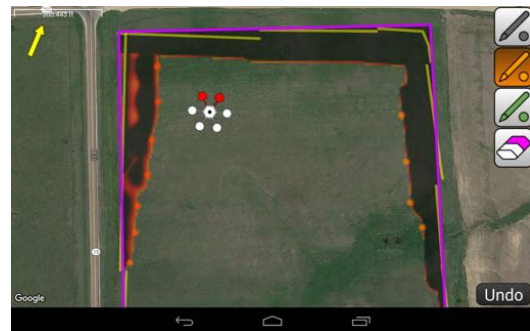
Fig. 9: The application interface the participants used to adjust the fire simulation. The tools for adjusting the fire simulation are on the right side. The black pen tool marks areas as burned, the orange pen tool marks areas as currently burning, the green pen tool marks areas as unburned, and the eraser tool erases marks.
