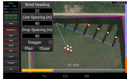
Fig. 3: UAS-Rx Android application for planning ignition lines. The UAS-Rx is represented as a red and white hexacopter on the satellite map. A pop-up menu over the map has inputs for the ignition planner. The grey line and blue dots are the planned path and ignition locations. The yellow slider serves to project the fire simulation into the future (set at 6 minutes in the future in the figure) and shows how the planned ignitions would connect to the previous ignitions.
